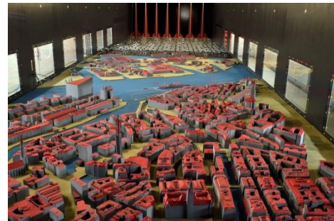
Fig.1 Wind tunnel model of Hamburg inner city
