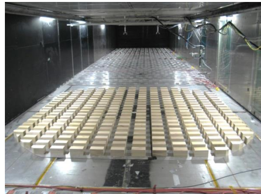
Fig.1 The DIPLOS array in the EnFlo wind tunnel
