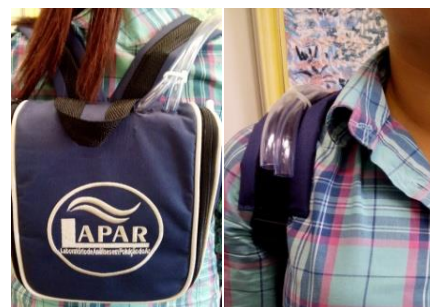
Fig.1 Backpack with the equipment for particulate matter measurements.
