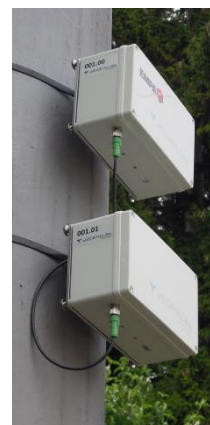
Figure 4: Aircube mounted at a utility pole in the city of Zurich.
