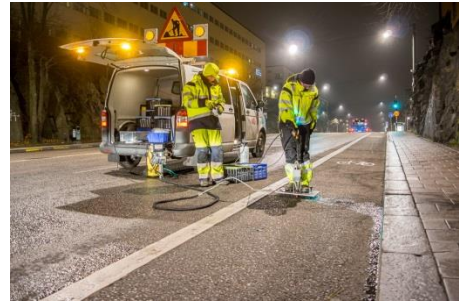
Fig.1 Sampling road dust load with Wet Dust Sampler
