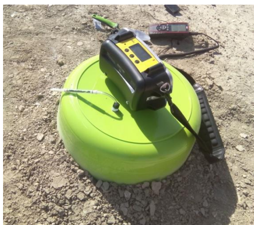
Fig.1 Measure of surface gas emissions with a flux chamber
