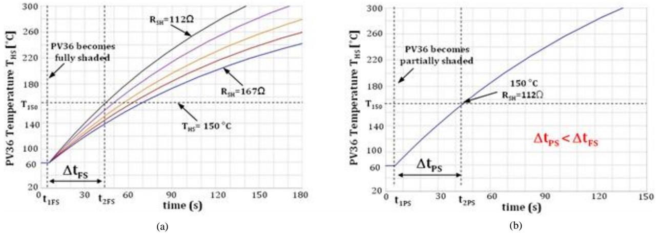
Fig. 7. Results obtained with our model for the behavior of the  $T_{HS}$  temperature of PV36 when: (a) PV36 becomes fully shaded after  $t_{IFS} = 5s$  ( $\gamma=0.01$ ) and for various values of  $R_{SH}$ ; b) PV36 becomes partially shaded after  $t_{IPS} = 5s$  (with  $\gamma=0.3$ ) and with the lowest value of  $R_{SH} = 112\Omega$  (worst case condition for the cell temperature).
