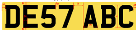
Fig. 3. GB number plate character format [13] including emblem, coachline, supplying outlet and BS identifier
