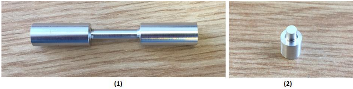
Figure 8.3.2 (1) A sample machined for microhardness and conductivity test and (2) section cut & polished for the microhardness test.
