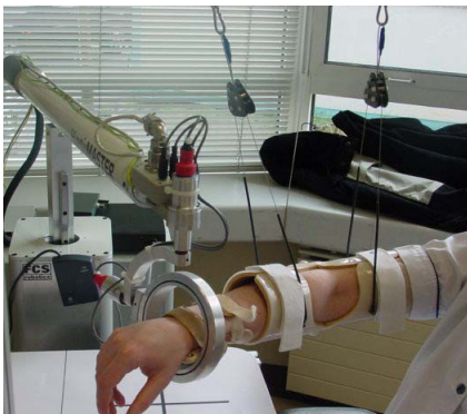
Figure 2.18: Elbow-orthosis used to de-weight patient's hand (Loureiro et al., 2001)
