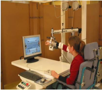
Figure 2.16: The GENTLE/S rehabilitation system (Amirabdollahian et al., 2007)
