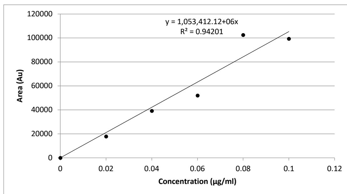
**Figure 36:** A calibration curve of concentration ( $\mu\text{g/ml}$ ) to area of the curve on the chromatogram (Au) for riboflavin and measured by HPLC with fluorescence detection (excitation and emission 450nm and 510 nm, respectively);  $y=1,053,412.12 + 6x$  .  $r^2=0.94$
