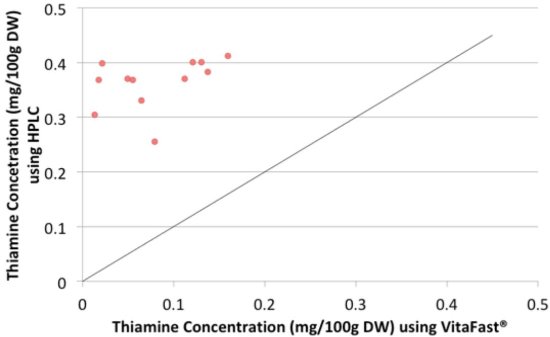
Figure 32: A scatter plot to show the agreement between the HPLC and Vitafast method when measuring thiamine in canned pulses using two methods on the same samples alongside total agreement of measurements shown by the line of identity. Regression analysis showed no proportional bias ( $p=0.727$ ).
