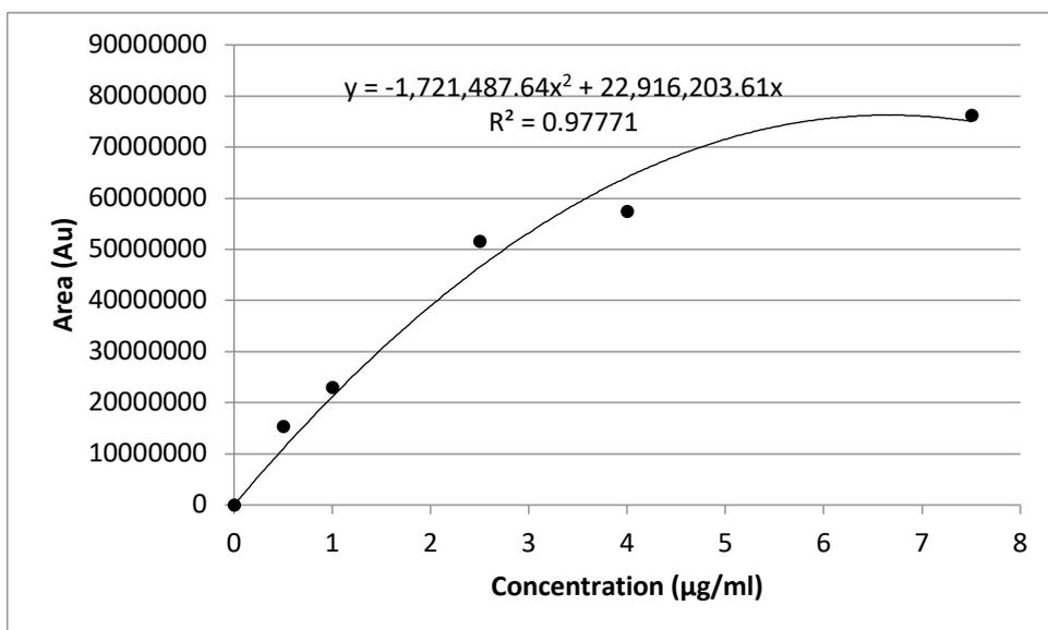
**Figure 30:** A calibration curve of concentration (mg/ml) to area of the curve on the chromatogram (Au) for derivatised thiamine hydrochloride to thiochrome and measured by HPLC with fluorescence detection (excitation and emission 360nm and 430 nm, respectively);  $y = -1,721,487.64x^2 + 22,916,203.61x$
