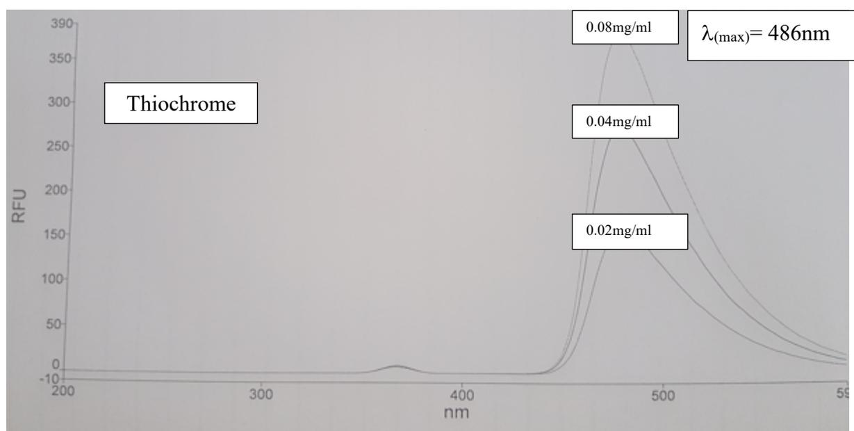
**Figure 29: A spectra of 0.08mg/ml, 0.04mg/ml and 0.02mg/ml thiamine hydrochloride derivatised to thiochrome measured on a fluorometer,  $\lambda_{(max)} = 486\text{nm}$ .**
