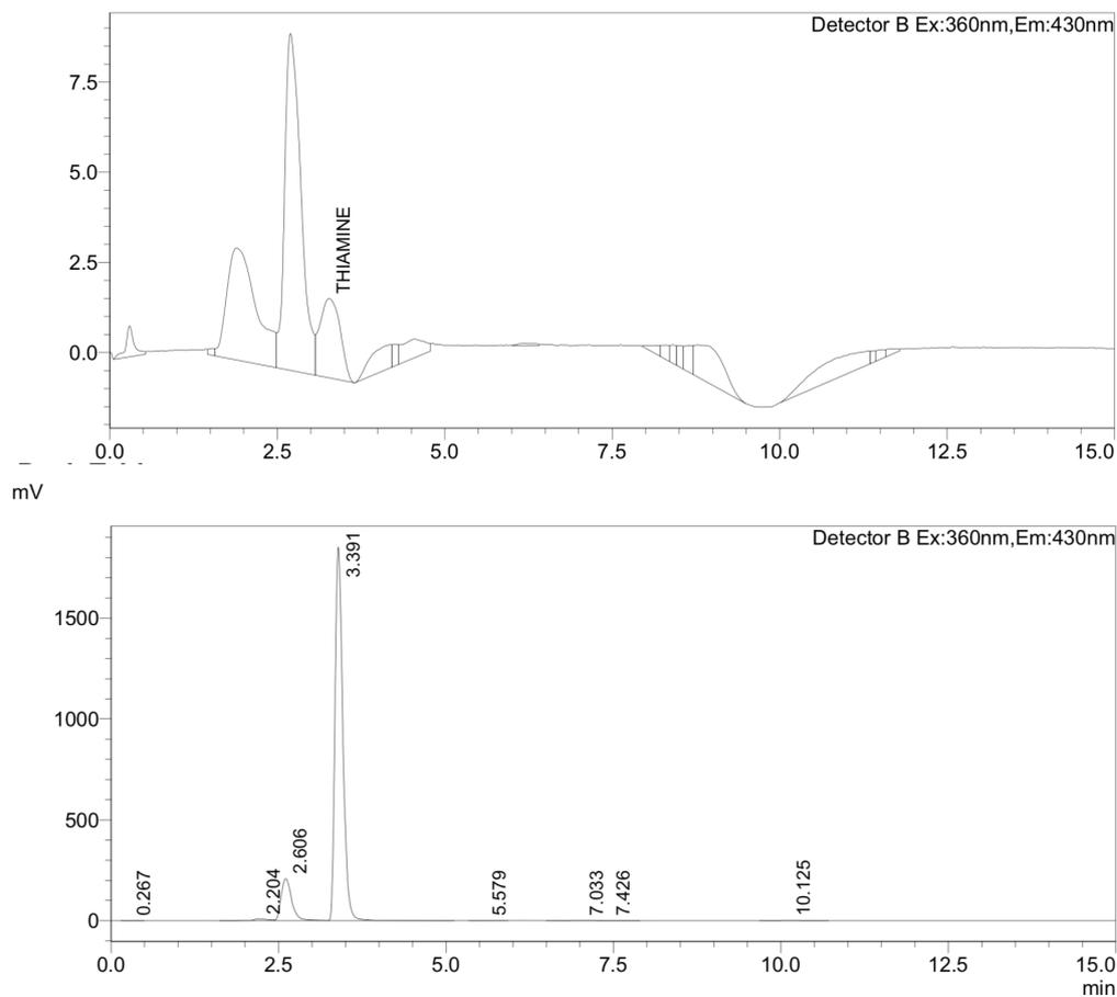
**Figure 35: The chromatogram for the limit of detection (LOD) for thiamine.**
