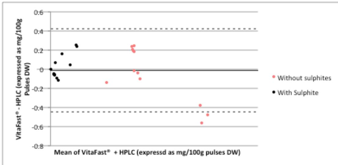
Figure 33: A Bland-Altman analysis plot to assess the agreement between the HPLC and VitaFast method when measuring thiamine in cooked sausages sodium metabisulphite. The ‘•’ identify those samples that contained sulphites. The ‘•’ identify those samples that did not contain sulphites. Bias =  $-0.013$ , 95% limits of agreement =  $[-0.447, 0.421]$  indicated by solid and dashed lines respectively. A one-sample t-test showed no significant difference between methods ( $p=0.781$ ).
