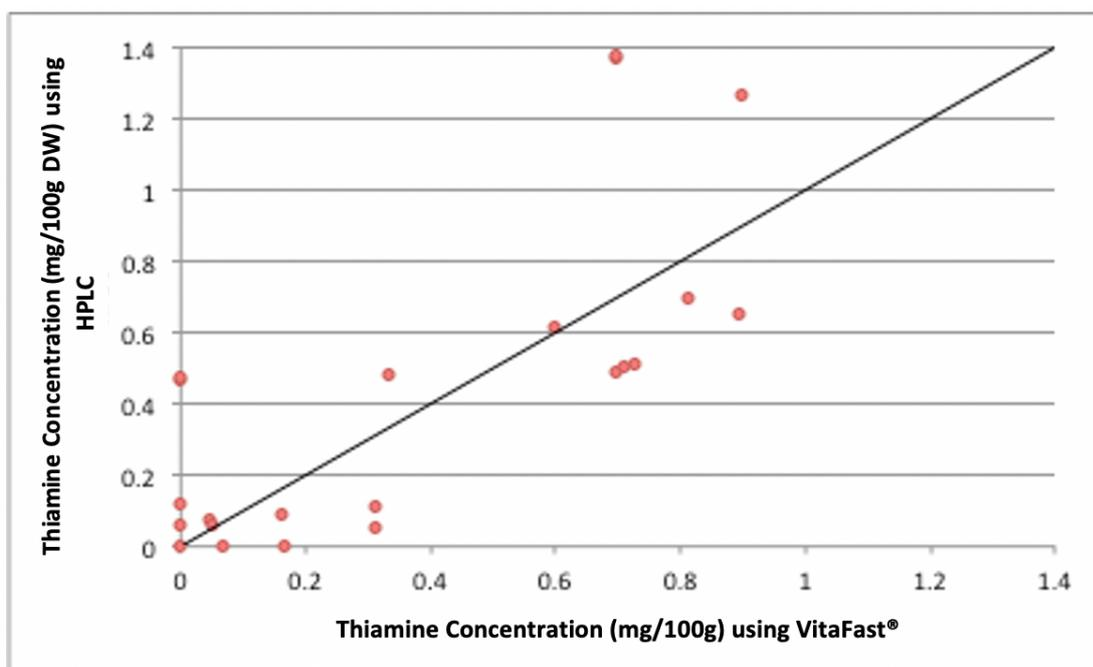
Figure 34: A scatter plot to show the agreement between HPLC and Vitafast method when measuring thiamine in cooked sausages using two methods on the same samples alongside total agreement of measurements shown by the line of identity. Regression analysis showed proportional bias ( $p < 0.05$ ).
