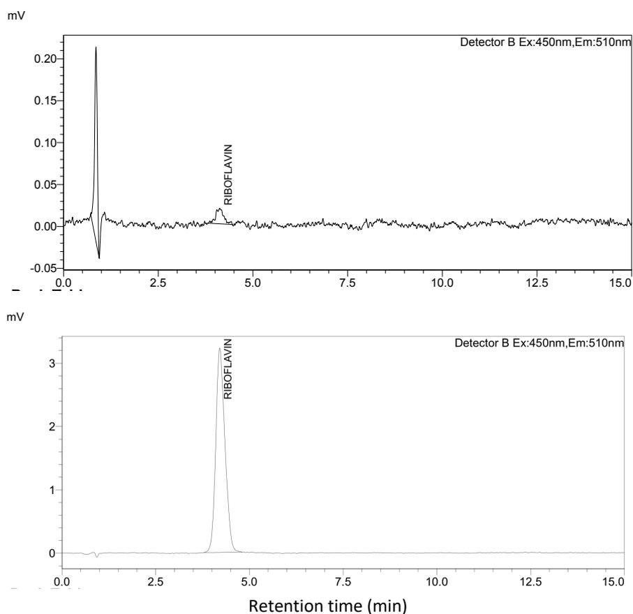
**Figure 46: Chromatograms of limit of detection (LOD) (top figure) and standard for riboflavin (bottom figure). The x-axis is the retention time and the y is mV.**
