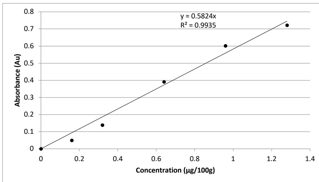
Figure 37: A calibration curve of concentration (µg/ml) to absorbance (Au) for folate read on a microtiter plate at 620nm;  $y=0.5824x$ .  $r^2=0.98$
