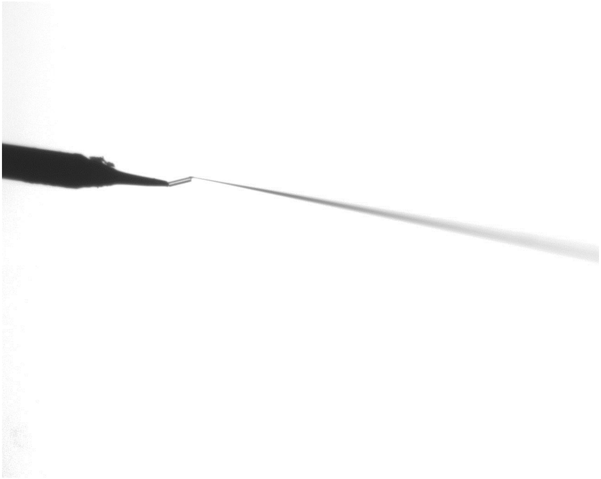
Fig. 4-19: Optical microscope image of an ice analogue crystal being attached to a glue-dipped sputter coated fibre at 4X magnification.
