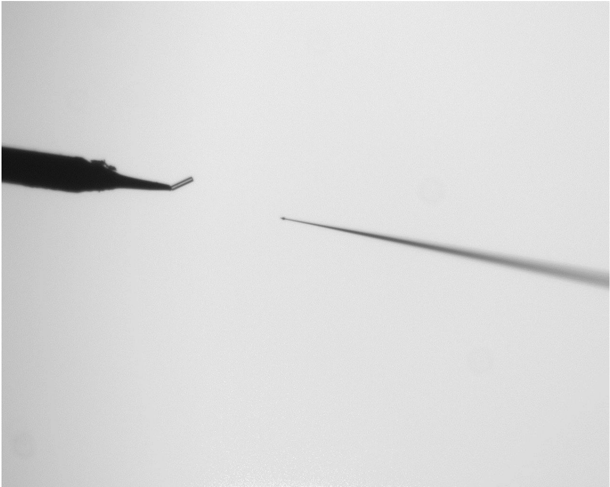
Fig. 4-18: Optical microscope image of a glue-dipped sputtered fibre and a probe-mounted ice analogue crystal at 4X magnification.
