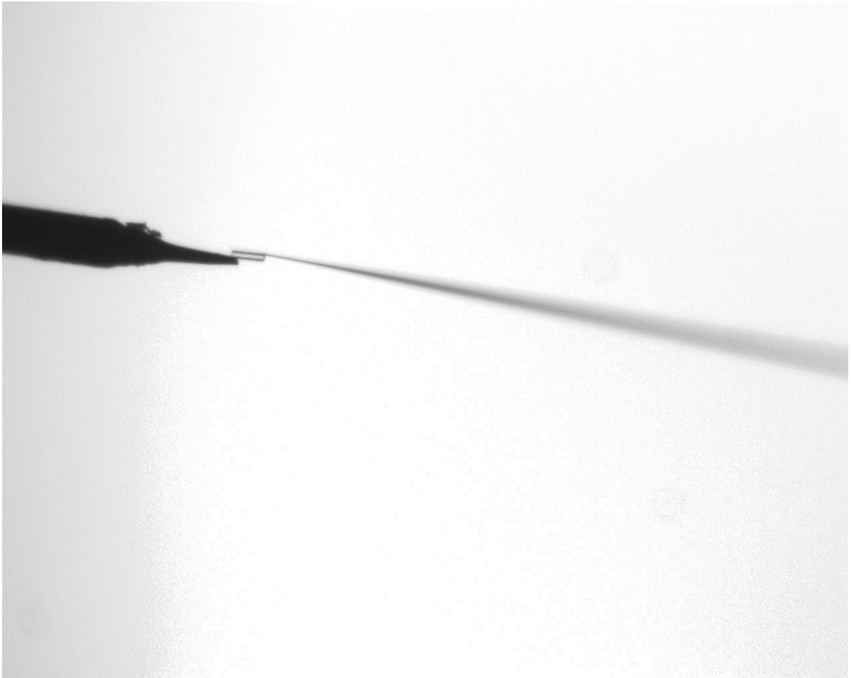
Fig. 4-20: Optical microscope image of an ice analogue crystal attached to a fibre with a probe being used to correct the crystal orientation at 4X magnification.
