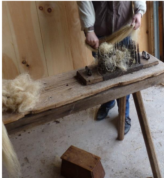
Figure 0.10, Author using heckle from the late eighteenth century. What will become the tear fibres are pulled through the heckle. The tow is left in the heckle.
