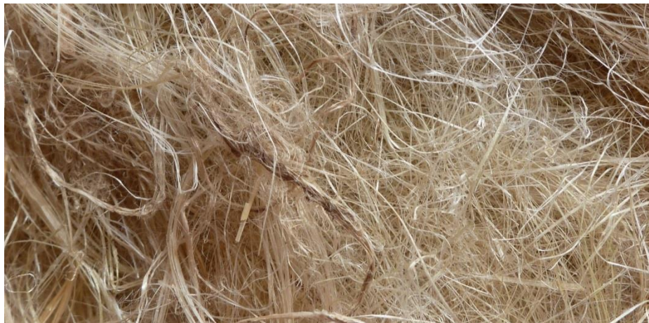
Figure 4.4, Tow fibre processed by the author. It has not been heckled further therefore the fibres are not aligned for spinning.
