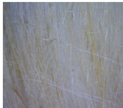
Figure 4.3, Williamsburg hemp fibre, microscope image, 60x magnification
