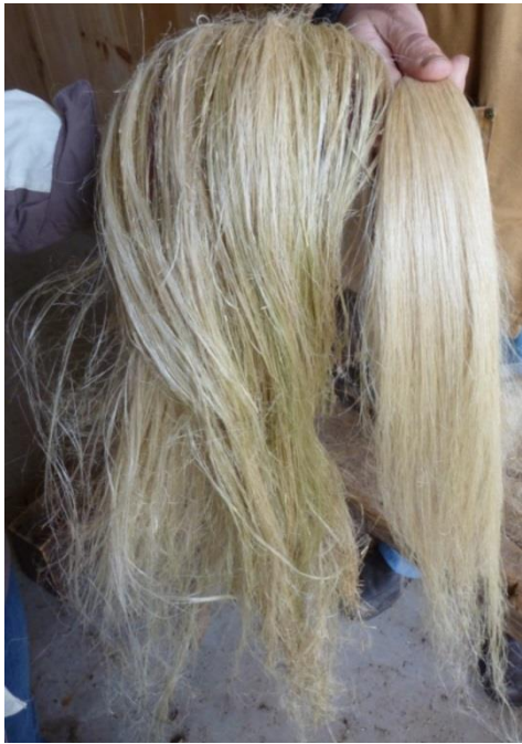
Figure 0.9, Scutched flax on the left, heckled flax on the right. This was the author's first attempt at scutching and braking therefore her scutched fibres are rougher and more matted than when worked by an expert.
