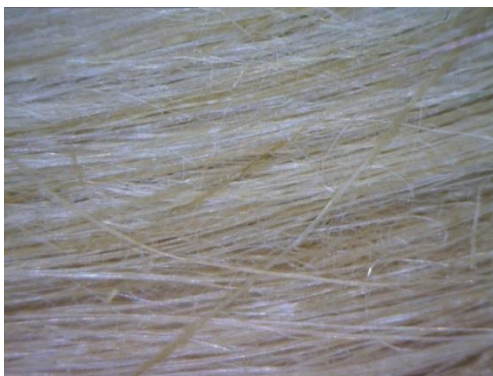
Figure 4.2, Williamsburg flax fibre, microscope image, 60x magnification
