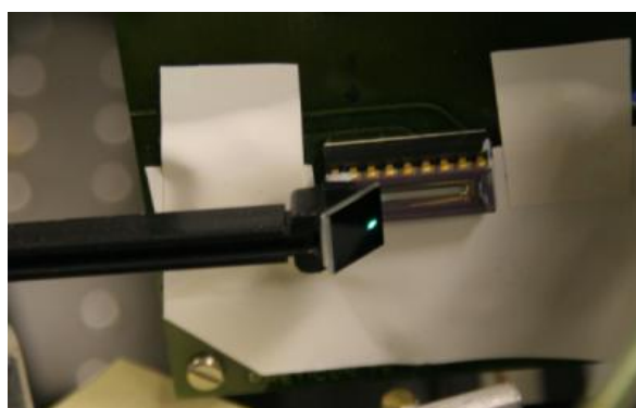
Figure 5-7 - Linear Photodiode Array used to capture small angle scattering data. The laser can be seen impacting on the mirror.
