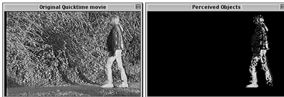
Figure 2: [Left] Real world pedestrian footage. [Right] The pedestrian is extracted using a combination of image preprocessing techniques, making the Active Contour’s task easier.
