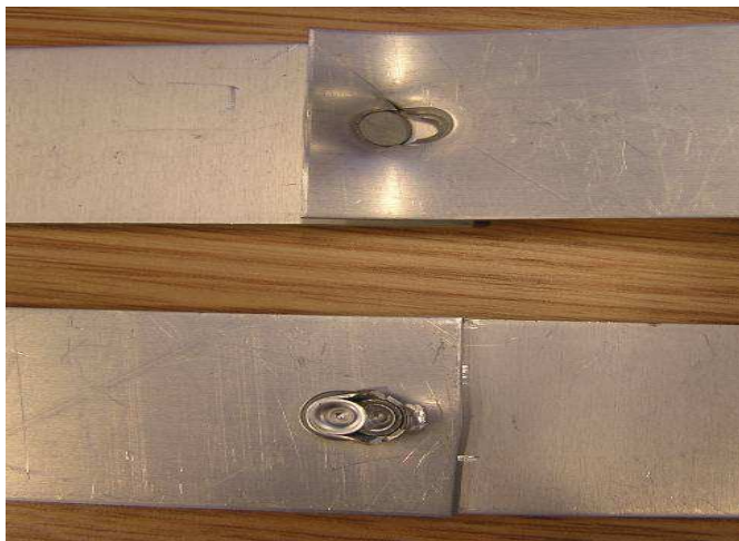
Fig.40 – Failure mechanism of Aluminium 5754 both configurations
