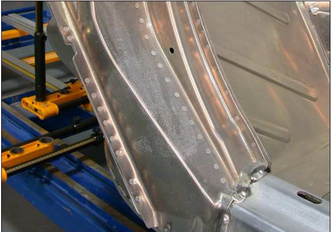
Fig.5 - The Chevrolet Corvette Z06 aluminium structure uses self-piercing rivets for assembling some stamped pieces together, for example the B-pillar
