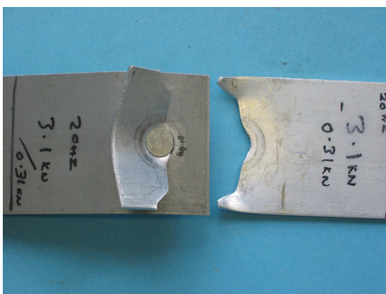
Fig.47b – Fatigue failure of (Aluminium 5182 top + IF steel bottom) joint configuration with 4.85 kN average shear strength
