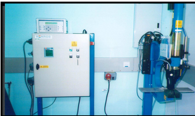
Fig.26 – Servo-electric self-piercing machine used for piercing the materials
