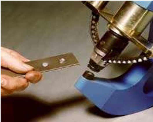
Fig.4 – High speed sheet joining process in which a semi-tubular rivet is set using a punch & die to flare the rivet within the lower sheet, no pre-existing hole is required
