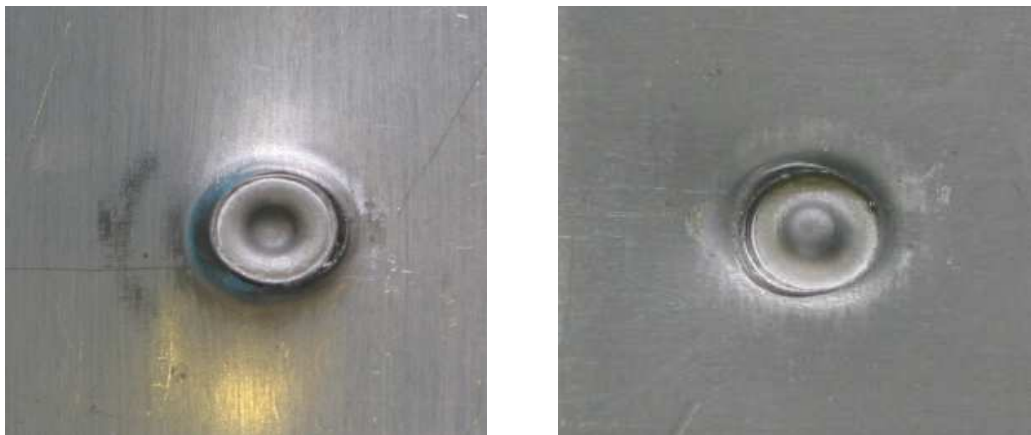
Fig.39 – Rivet pull-out of 1.5mm Al5182 on top + 1.2mm I.F. steel on bottom
