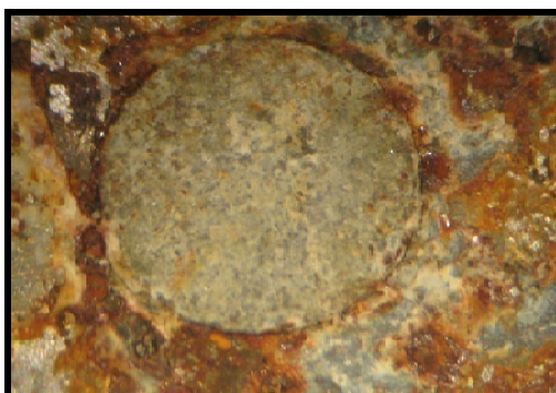
Fig.76d – SPR after 845 hours of exposure
