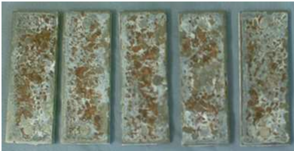
Fig.77 – Significant amount of zinc which had been lost from the I.F. steel surface after 660 hrs
