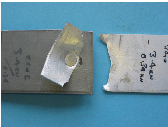
Fig.47a – Fatigue failure of (Aluminium 5182 top + IF steel bottom) joint configuration with 4.85 kN average shear strength
