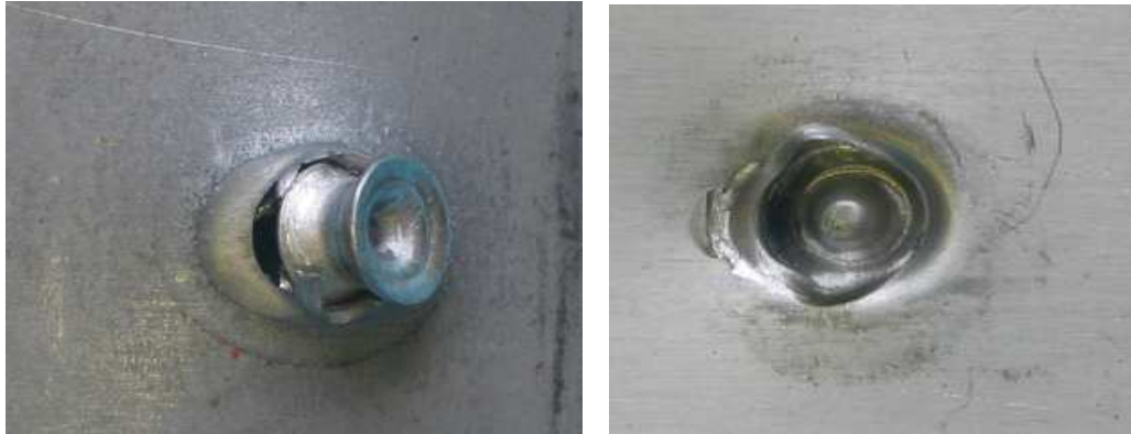
Fig.38 – Rivet pull-out of 1.2mm I.F. steel on top + 1.5mm Al5182 on bottom
