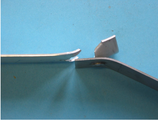
Fig.47c – Substantial bending of both Aluminium 5182 and I.F. Steel
