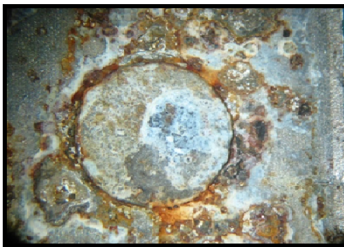
Fig.76c – SPR after 660 hours of exposure
