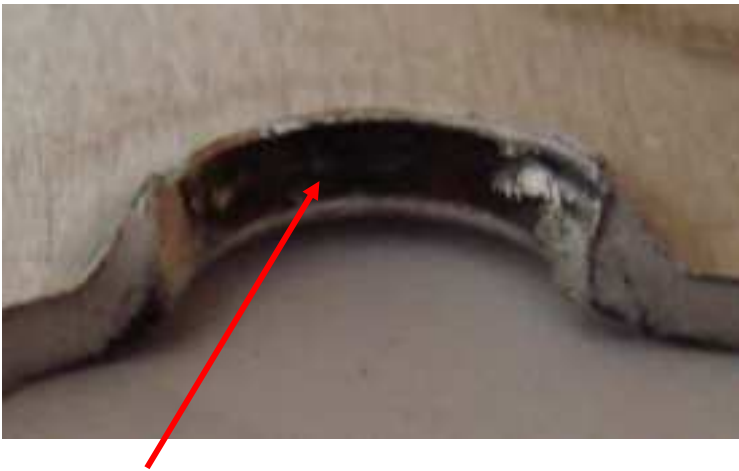
Fig.63 – Fretting scars at the periphery of the buttonhole of the Al 5182
