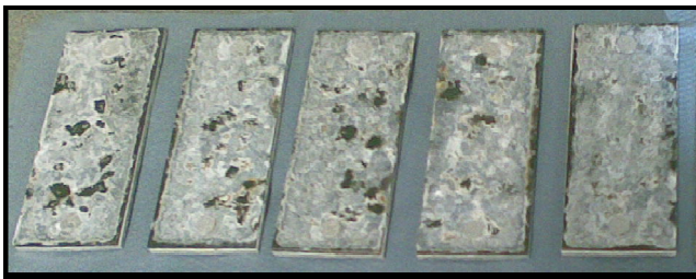
Fig.70 – Samples after 187 hrs of corrosion treatment
