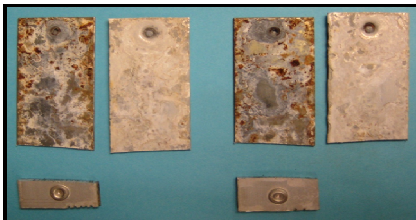
Fig.72 – Progression of the corrosion progressing towards the centre of the overlap after 660 hrs of corrosion
