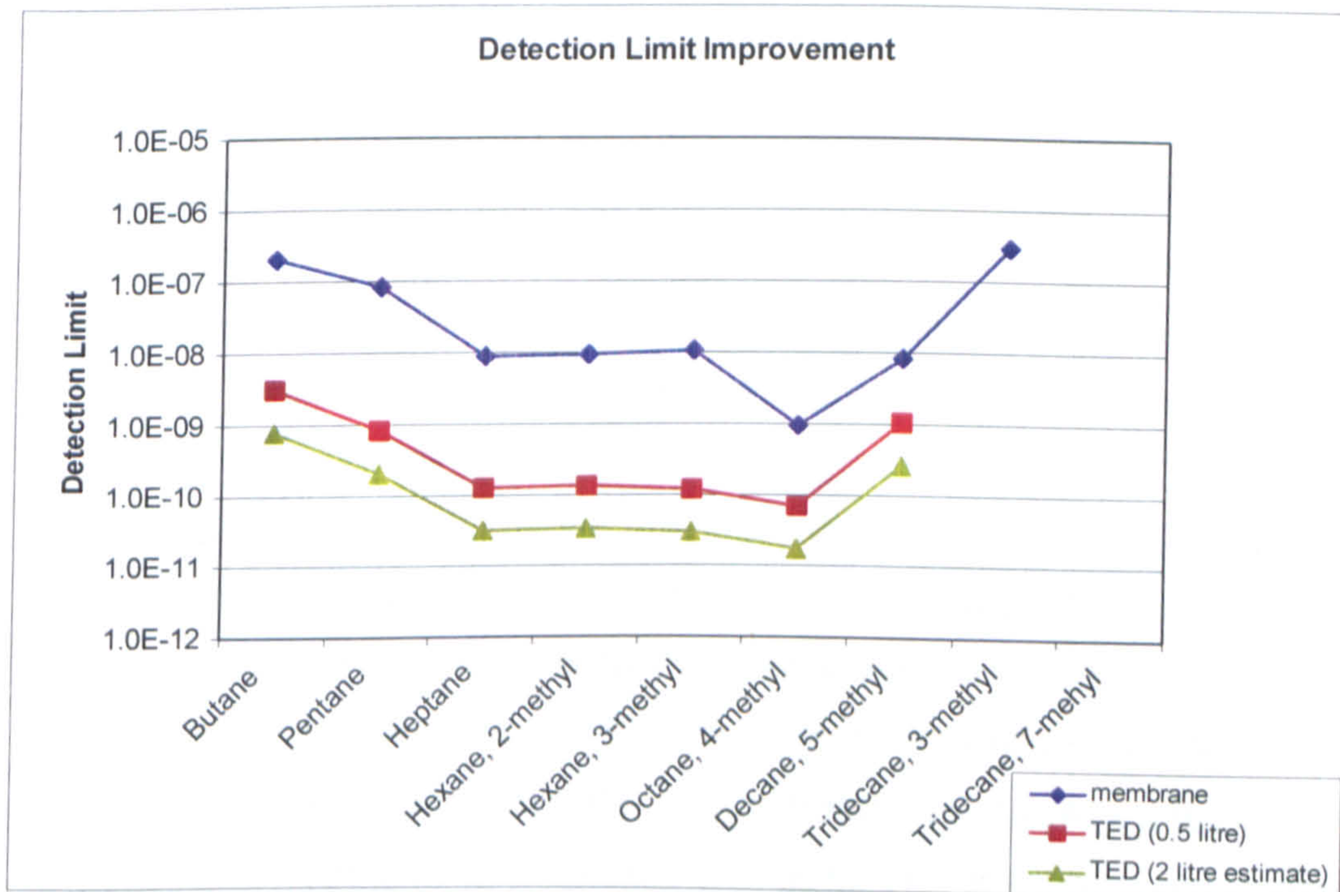
Figure 52: Detection Limit and Sensitivity Comparison between double membrane and TED
